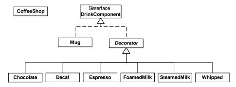
Methods invoked on the Decorator can in turn invoke methods in the component, and can of course perform processing before or after the invocation.
