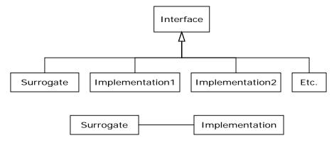
When a surrogate object is created, it is given an implementation to which to send all of the method calls.
