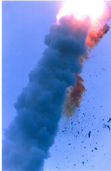
Figure 4: Ariane explosion was caused by buffer overflow
