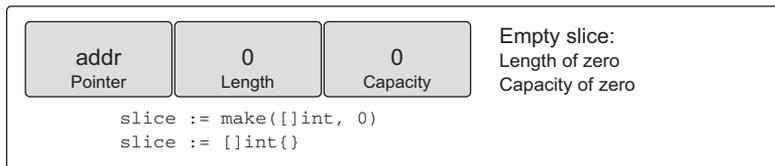
Figure 4.11 The representation of an empty slice
