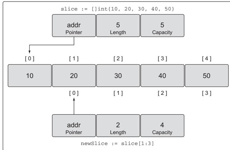
**Figure 4.12** Two slices sharing the same underlying array
