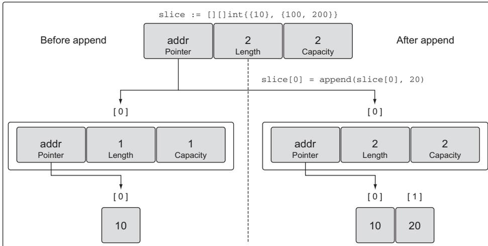
**Figure 4.21** What index 0 of the outer slice looks like after the `append` operation
