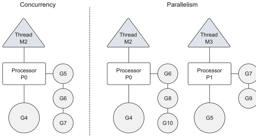
Figure 6.3 Difference between concurrency and parallelism
