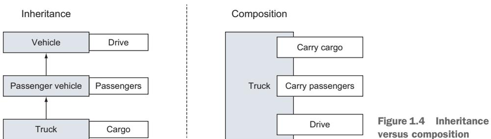
**Figure 1.4** Inheritance versus composition
