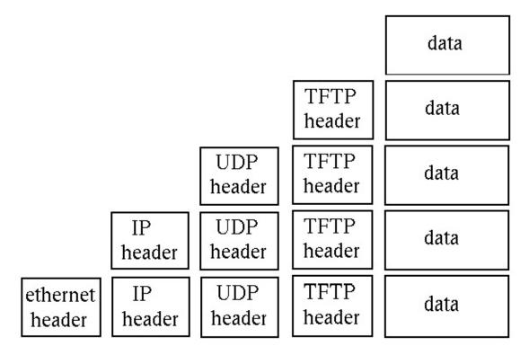
The packet transmitted over ethernet, is of course the bottom one.
