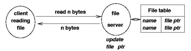
In NFS, the server does not maintain this state. The client does. Each file access from the client that reaches the server must open the file at the appropriate point, as given by the client, to perform the action.
